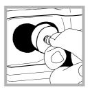
4. For safety, insert one of the the plastic covers (supplied with your machine) over the hole.
